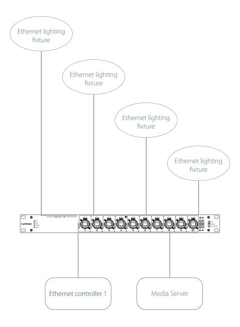
In this example, users wishes to control all Ethernet lighting fixtures from both the Ethernet controller and the media server. This means all fixtures will receive two different control streams, such as Art-Net ones. As lighting fixtures are not equipped to merge Art-Net streams, they'll all be confused, resulting in a strange and random behavior.
