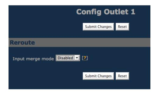
By using the drop down menu, you can select here to merge the incoming DMX with the converted protocol using either HTP or LTP policy. Don't forget to submit changes! Once all your **reroute** settings are made, don't forget to submit changes on the main page.
