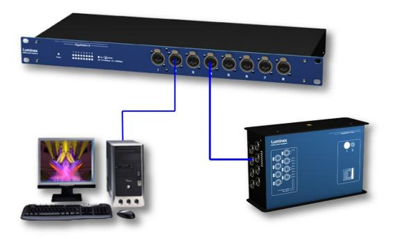
The link/Act LED for each UTP port blink turns green when the link is valid. A flashing Link/Act LED indicates packet activity on that port. A LED on the bottom indicates a port speed of either 10/100Mbps or 1000Mbps (see Illustration 1).
