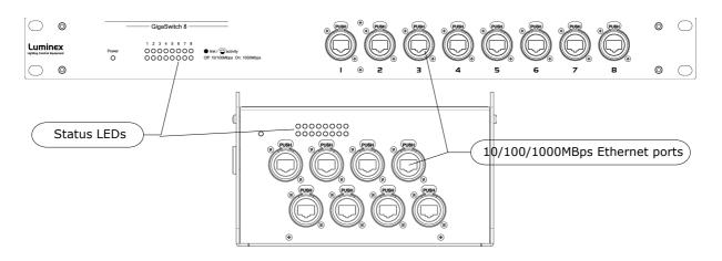
8 X shielded Ethercon connectors (rack version default configuration)
