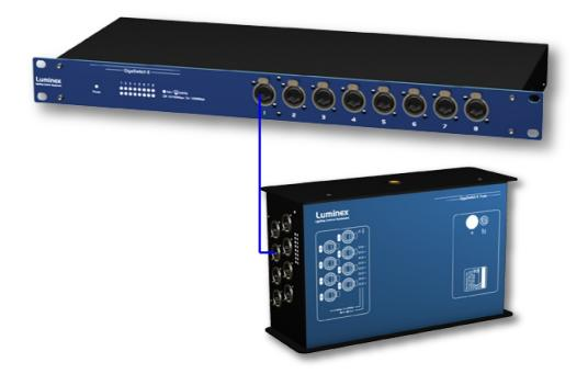
The hub or switch can be connected to the GigaSwitch 8 using either a straight cable or crossover cable; any cable is fine. The GigaSwitch 8 comes with the MDI/MDIX feature.
