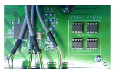
2 DMX transceivers and 2 optical couplers are provided to replace the ICs of a permanently broken DMX outlet.
