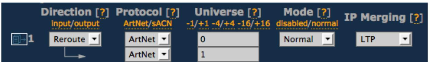
First, we select **reroute** in the direction field. Then we set the incoming protocol as Art-net, on universe 0. This means both the controller and the media server must use universe 0, to control the fixtures. Then we enable the LTP IP merging. This means all universe 0 coming from the network will be merged following LTP policy. Then, the result of this merge will be converted to Art-Net universe 1.
