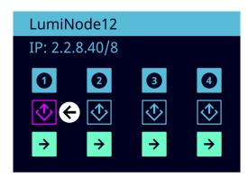
If the port is in DMX redundant mode and active the output icon is solid magenta: 💇
