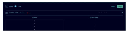
You can define the control channel, the protocol and universe number, as the IP address of the control source. Click on the gear wheel icon to change these parameters.
