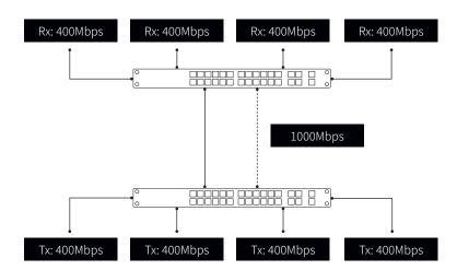
However, only one link is active between the switches, as the other link is used as redundant link. So, a maximum of 1000Mbps data transfer can be achieved on this link. In our example, we need 1600Mbps of throughput to transfer all four video streams between the switches. This is not enough, the link between the switches will create a bottleneck, resulting in data loss or data delay. The video streams won't be delivered in time and will create lag in the video output.
