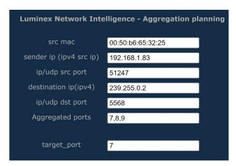
According to the parameters of your Ethernet frame, the page will show you which port will be in use. This allows you to predict, but also to solve some problems. In the unlikely event of an overloaded link in an aggregation, the user can solve the problem by simply changing the appropriate IP address for the source, for example.
