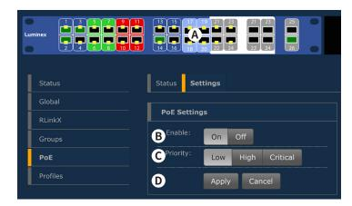
The priority of a port is used when the switch reaches the limit of its maximum output power. In the unlikely situation of the PoE devices requiring too much power from the switch, the switch will first disable the port(s) with the lowest priority.
