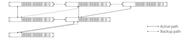
If one of the active paths fails, the switches will enable a redundant path in a seamless manner.
