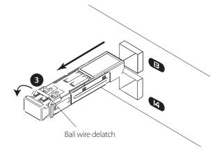
3 Open the bail wire to disengage and remove the mini-GBIC transceiver.
