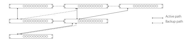
To create a redundant path with RLinkX, simply connect a minimum of two links between two GigaCore switches. The blue RLinkX LEDs of the connected ports will turn on, indicating the redundancy is active and available.
