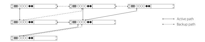
To create a redundant path with RLinkX, simply connect a minimum of two links between two GigaCore switches. The blue RLinkX LEDs of the connected ports will turn on, indicating the redundancy is active and available.
