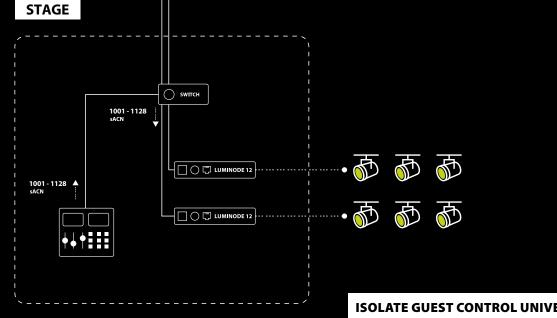
The main house controller(s) and the lighting rig is controlled via universe 1001 – 1128 (128 universes). All the guest consoles are isolated from the rig by sending out universe 1-128. The main console is setup as trigger source to switch between the different guest sources coming in on the LumiCore and defining who can control the rig (and even which part if split in different trigger channels).
