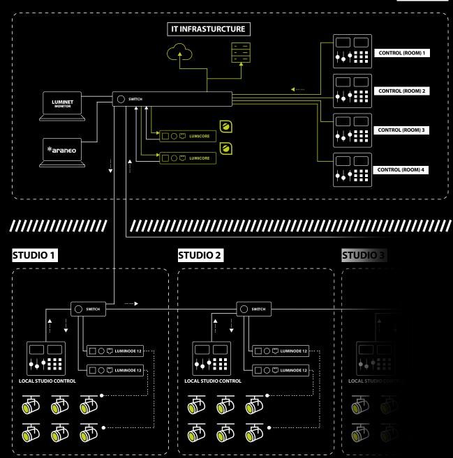
With its split interface possibilities LumiCore allows you to isolate your lighting rig LAN from the IT infrastructure. This allows you to monitor your control infrastructure from the IT department
